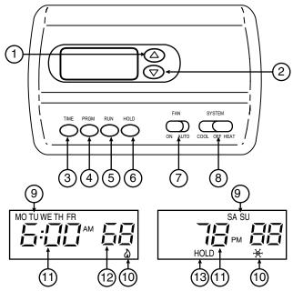
Figure 8. Thermostat display, buttons, and switches
